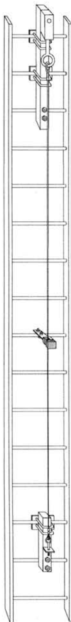
Components Mounted on Ladder with Cable
